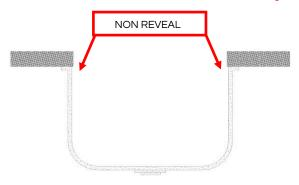
A non positive reveal is the most common and preferred application - where the countertop extends over the edge of the sink rim on all sides.
