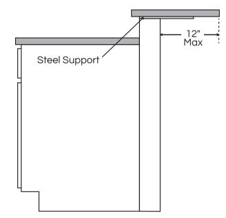
Tabletop application requires the use of a full substrate which extends within 4" of the edge of the table top. The manufacturer's specification for the pedestal must be checked to verify it is designed to support the size and weight of the table top.
