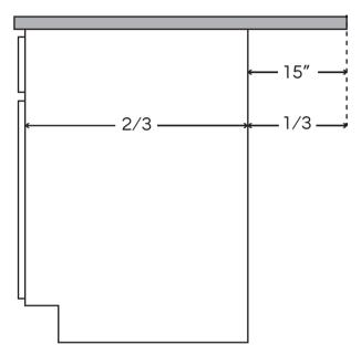
Overhang greater than 15" requires corbels or flush mounted steel supports. Supports must be designed to bear the weight of the countertop and be mounted to studs or equivalent load bearing structure. Supports can bear no more than 24" of overhang. Maximum 36" between centers of each adjacent support.
