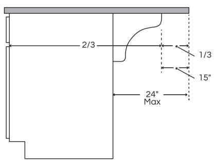
Overhang that exceeds 24" requires the use of substrate and posts installed evenly at a maximum of 36" between centers of each adjacent support. Tops on half wall can be installed using steel supports with overhang up to 12". Overhang greater than 12" will require corbels or legs.
