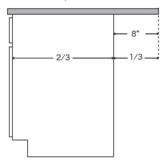
Overhang greater than 8" requires corbels or flush mounted steel supports. Supports must be designed to bear the weight of the countertop and be mounted to studs or equivalent load bearing structure. Supports can bear no more than 24" of overhang. Maximum 36" between centers of each adjacent support.
