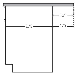
Overhang greater than 12" requires corbels or flush mounted steel supports. Supports must be designed to bear the weight of the countertop and be mounted to studs or equivalent load bearing structure. Supports can bear no more than 24" of overhang. Maximum 36" between centers of each adjacent support.
