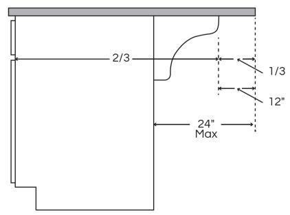
Overhang that exceeds 24" requires the use of substrate and posts installed evenly at a maximum of 36" between centers of each adjacent support.
