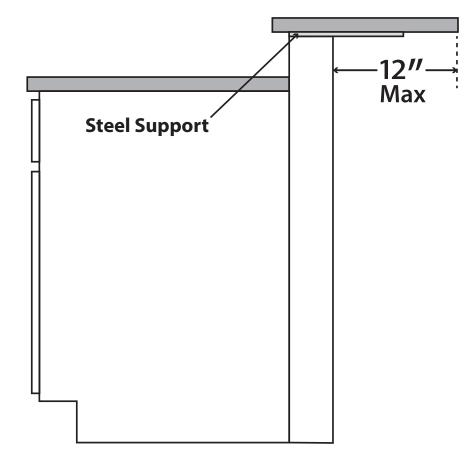
Tabletop application requires the use of a full substrate which extends within 4" of the edge of the table top. The manufacturer's specification for the pedestal must be checked to verify it is designed to support the size and weight of the table top.
