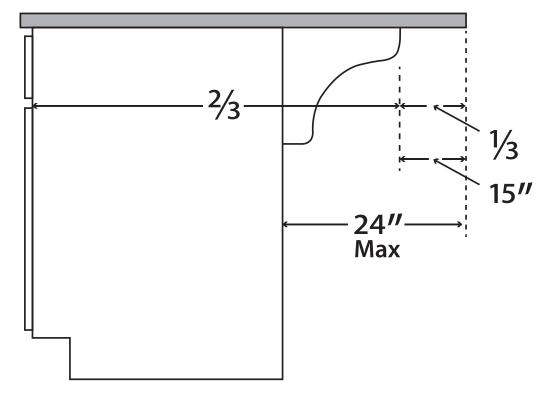
Overhang that exceeds 24" requires the use of substrate and posts installed evenly at a maximum of 36" between centers of each adjacent support.
