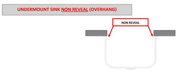
A non positive reveal is the most common and preferred application - where the countertop extends over the edge of the sink rim on all sides.
